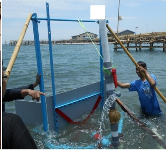
Fig. 4.1. Energy conversion plate on the suction position
