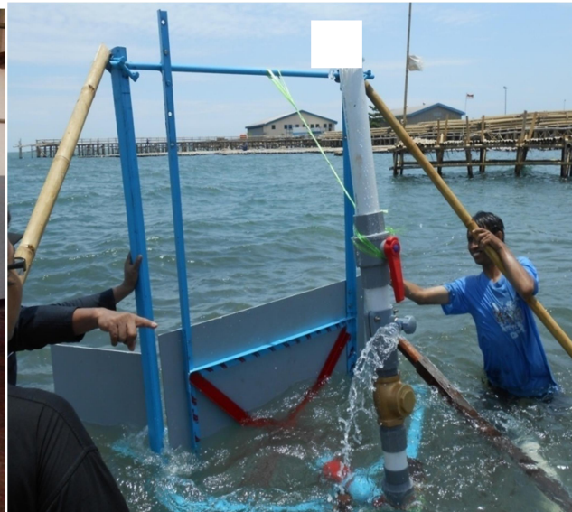
Fig. 4.1. Energy conversion plate on the suction position
