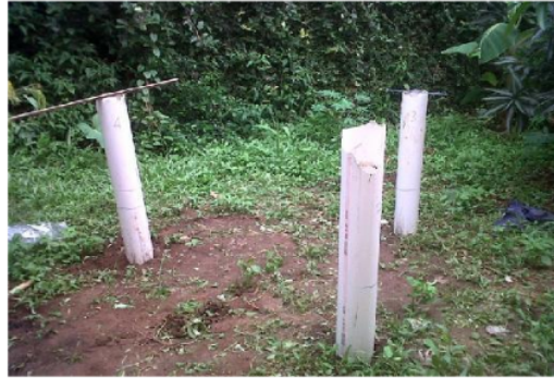
Figure 2. Configuration of Bio Pore Infiltration Hole for finding in-situ permeability coefficients
