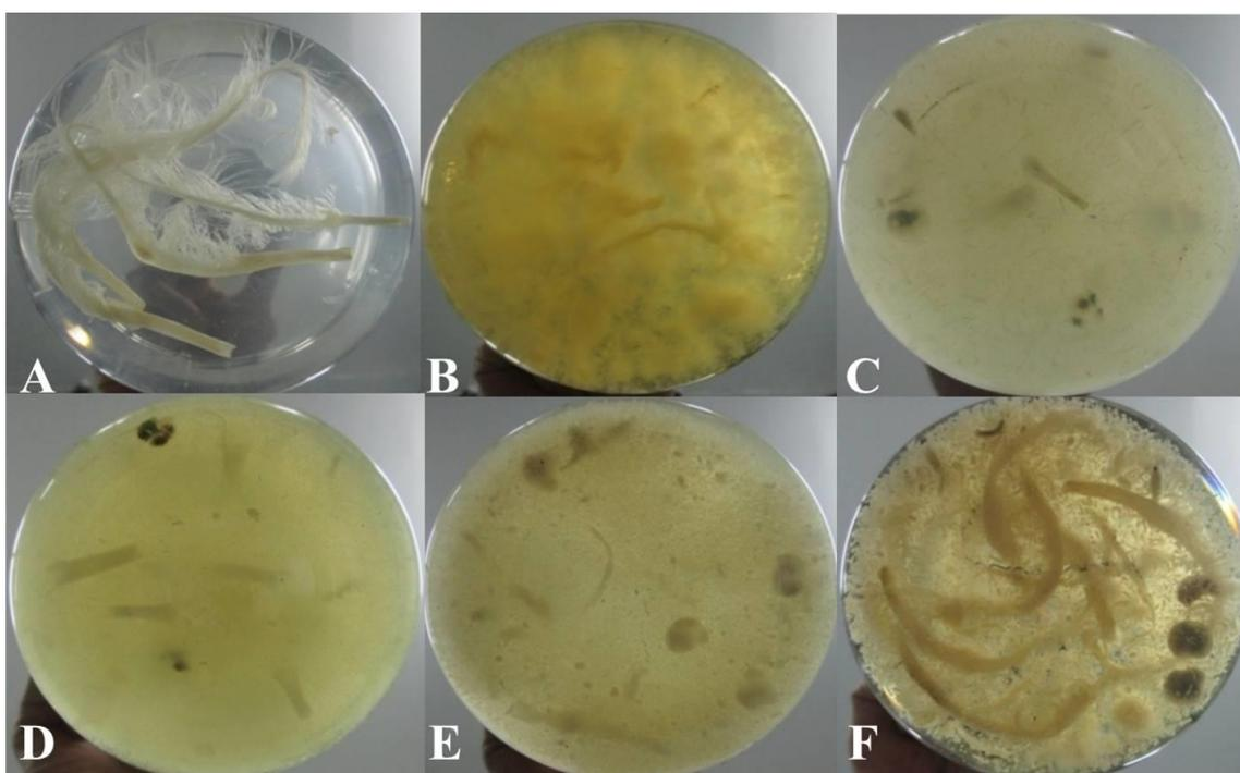
**Fig 3** – Biodegradation Test Result of Chicken Feathers Waste after 10 Days Incubation. A Control. B Treatment on Isolate A29. C Treatment on Isolate K18. D Treatment on Isolate A18. E Treatment on Isolate A12. F Treatment on Isolate K2.
