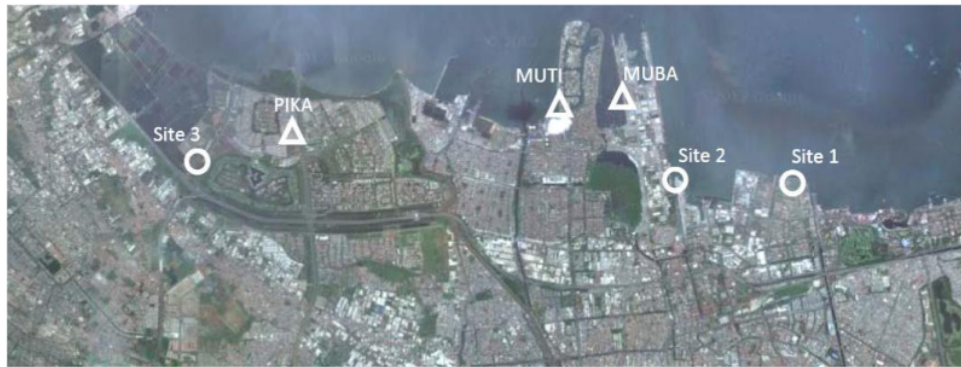
Figure 1. Land Subsidence measurement using GPS in part coastal areas of Jakarta (Source: Abidin, 2008)
