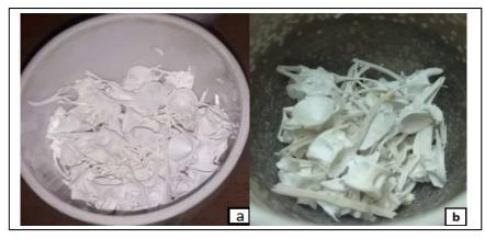
Fig. 3. CaO results from calcination of Tuna Bone at a temperature of 1000 °C(a). For 6 hours (b). For 10 hours
