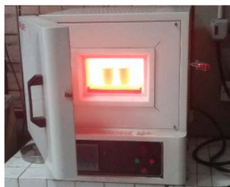
Figure 1. Calcination process with a temperature of 1000°C
