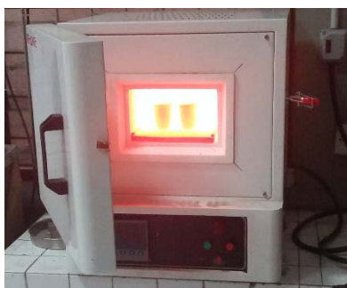
Figure 1. Calcination process with a temperature of 1000°C
