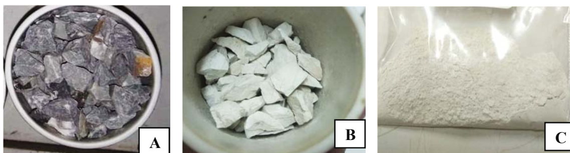
Figure 2. Limestone (a) Before calcination (b) Aftercalcination (c) After digerus
