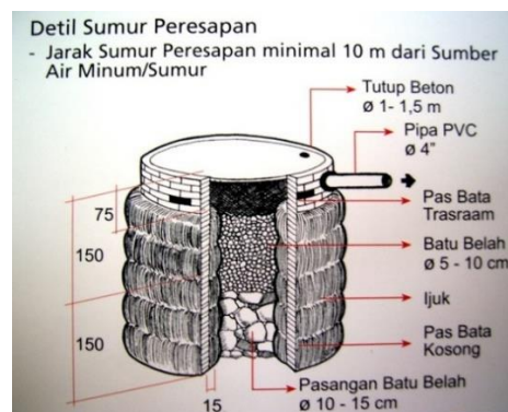
Detail Sumur Resapan
