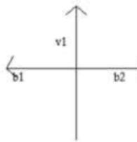
$$\begin{aligned}\Sigma V &= 0 \\ V1 &= 0 \\ \Sigma H &= 0 \\ -b1 + b2 &= 0 \\ b2 &= +1167,14 \text{ kg (Batang tarik)}\end{aligned}$$
