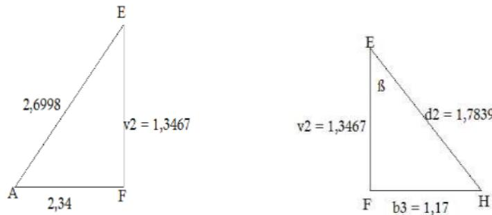
$$\begin{aligned}\sin \beta &= \frac{b_3}{d_2} = \frac{1,17}{1,7839} = 0,65586636022 \\ \beta &= 40,98537466175^\circ\end{aligned}$$
