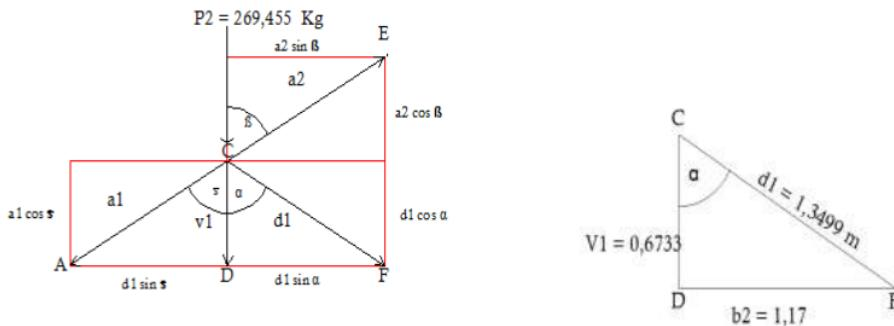
$$\begin{aligned}\sin \alpha &= \frac{b^2}{d_1} \\ &= \frac{1,1700}{1,3499}\end{aligned}$$
