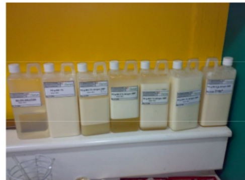
Fig. 6. Separation of PE-g-MA after cooling
