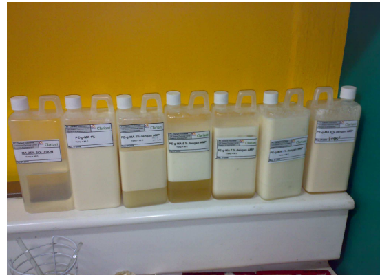
Fig. 6. Separation of PE-g-MA after cooling
