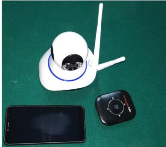
Gambar 2. IP camera, Smartphone dan Router CDMA
