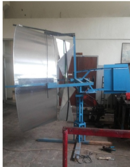
Fig 2.2. Installed wind turbine with cone tunnel
