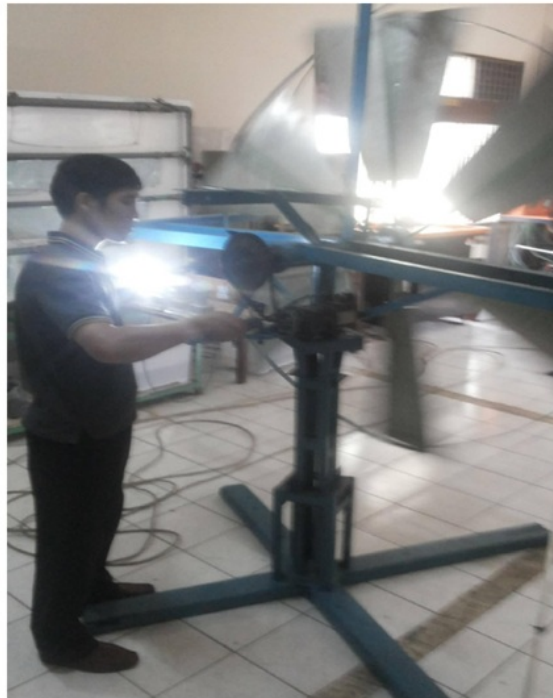
Fig 3. Measurement of rotation speed generator
