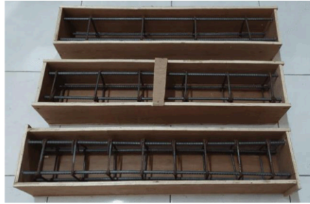
Figure 7. The assembled specimens of reinforced concrete beams with formwork are ready for casting
