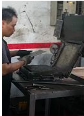
Placement of the steel plate on the mould
