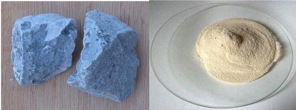
Gambar 42 . Kalsium Karbida ( $CaC_2$ )
