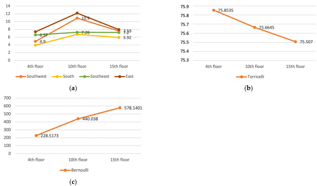
Figure 9. Comparison of the field calculations and measurements: (a) Air velocity from the field measurement; (b) Torricelli equation; and (c) Bernoulli equation.
