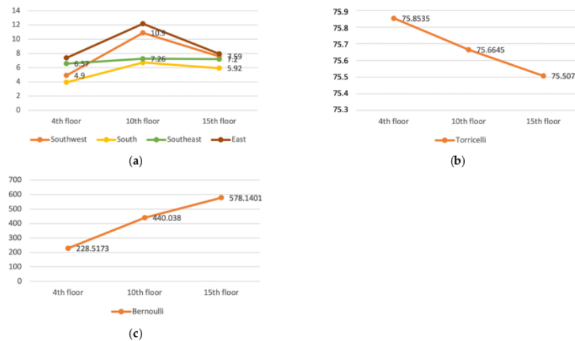
Figure 9. Comparison of the field calculations and measurements: (a) Air velocity from the field measurement; (b) Torricelli equation; and (c) Bernoulli equation.
