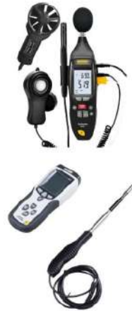
Figure 2. Environment Meter and Hot Wire Anemometer
