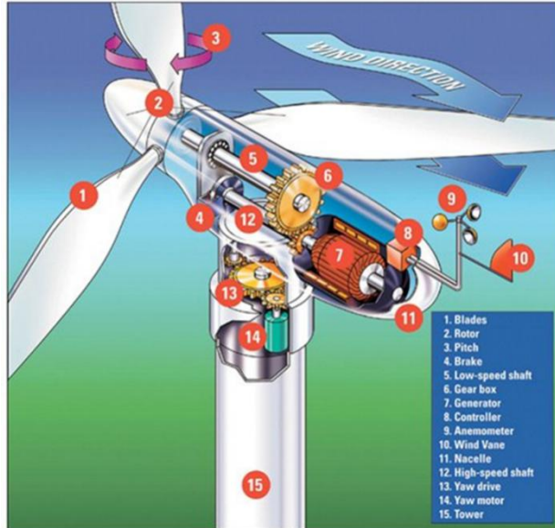
Fig. 2.2 Bagian-bagian PLTB (sumber: http://voyagesscolaires.lttt.lu/wp-content/uploads/2014/06/img10.jpg )
