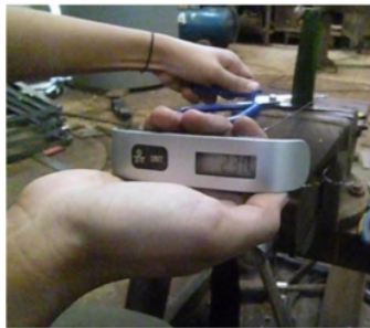
Figure 6. Measurement of friction by scissor method.
