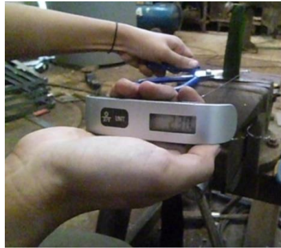
Figure 6. Measurement of friction by scissor method.
