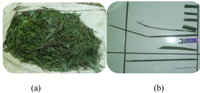
Figure 9. Size reduction of leaves by combine machine blades (a) mixed cuttings (b) cutting size variation.
