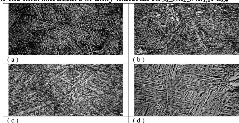
**Figure 4.2** Photogram  $Zr_{96,2} Sn_{2,3} Nb_{1,1} Fe_{0,4}$  alloy material surface with magnification of 500 X: (a) the original sample (not heat treatment), after the heat treatment (b)  $500^\circ C$ , (c)  $600^\circ C$ , and (d)  $700^\circ C$ .
