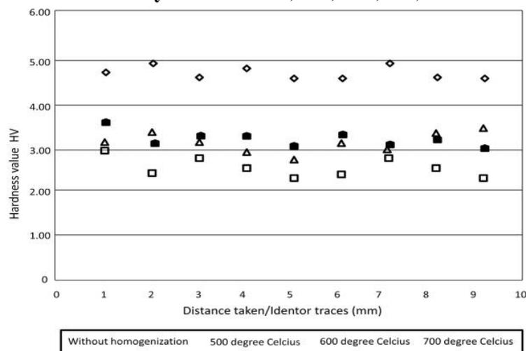
**Figure 4.3** Hardness Test Results on alloy material  $Zr_{96,2}Sn_{2,3}Nb_{1,1}Fe_{0,4}$
