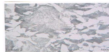
Figure 7. Micrograph basic material in the form of ferrite (white) and pearlite (black). E6013
