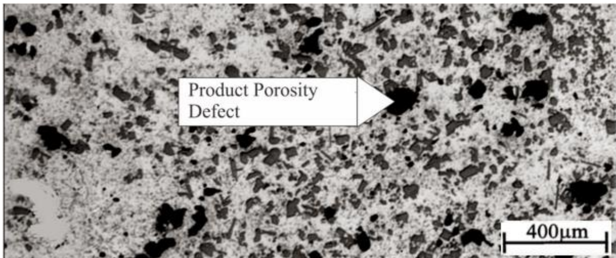
Figure 8. ADC-12 alloy LOM micrograph with overflow system.
