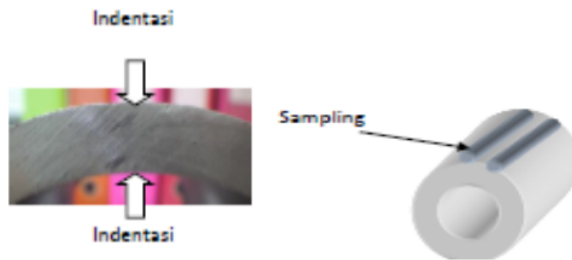
Figure 3. Position of sample hardness testing.
