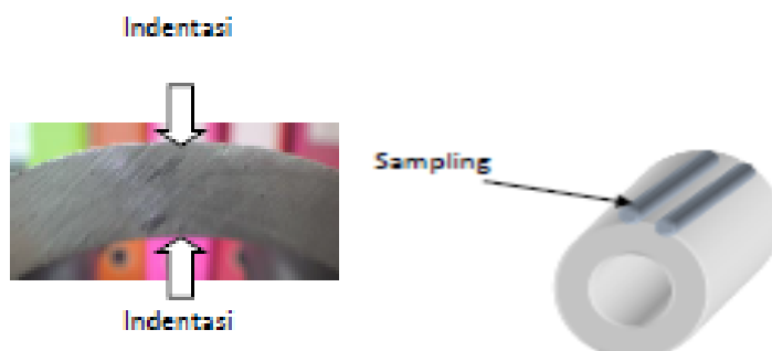
Figure 3. Position of sample hardness testing.
