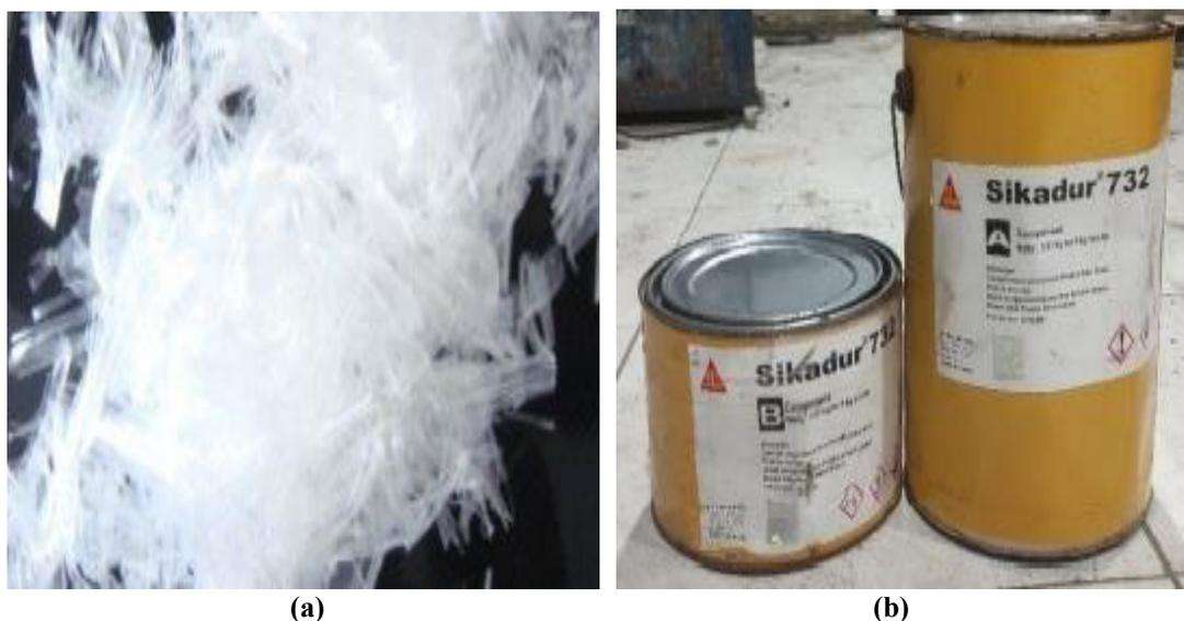
Gambar 1. (a) Material Aditif Polypropylene Fibre Mesh (PFM); (b) Epoxy Resin
