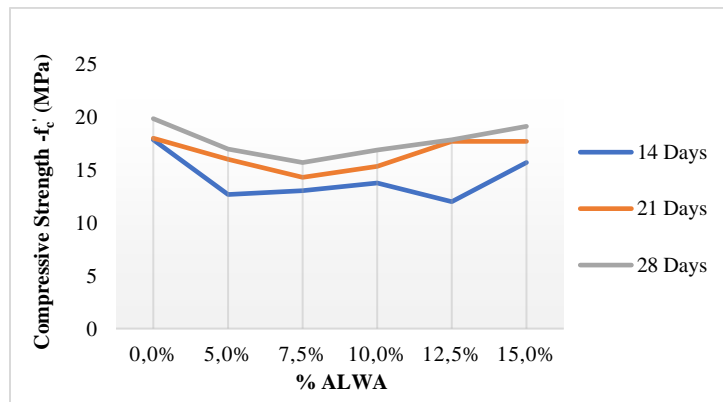
FIGURE 5. Compressive strength of 12.5% fly ash mixed concrete with a variation of ALWA addition
