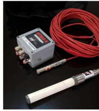
Figure 3. Piezometric Instrument and Data Logger Set
